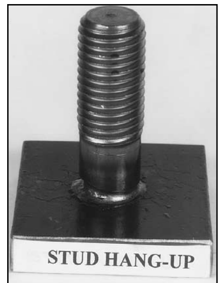
Fig. 12. Visual inspection of stud weld appearance. Source: Nelson Stud Welding, Inc.
